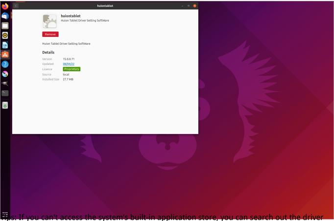
Files: If you can't access the system's built-in application store, you can search out the driver file, huiontablet\_xxx.deb, then double-click it to enter the installation interface, and click the remove button to uninstall it.
