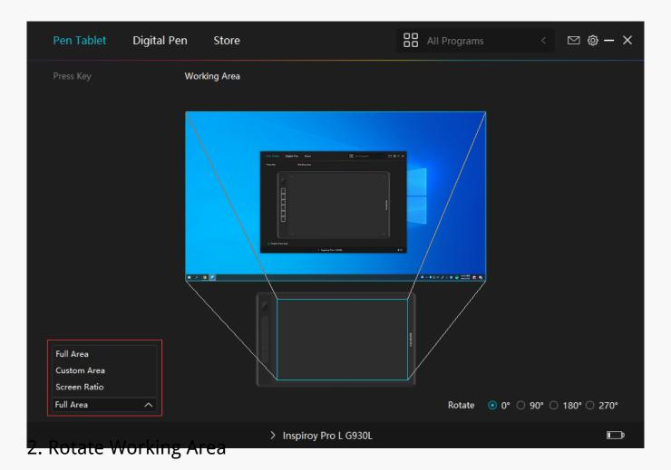
By changing the direction of the tablet to adapt to the left and right hand operation. You can rotate the tablet by  $0^{\circ},90^{\circ},180^{\circ}$  or  $270^{\circ}$ .
